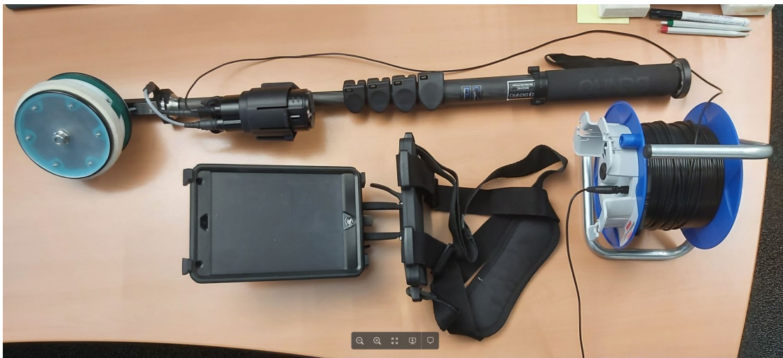
Figure 8 : PM8500 One wheel electrode cabling set up
