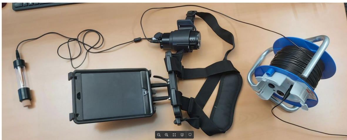
Figure 7 : PM8500 Rod electrode cabling set up
